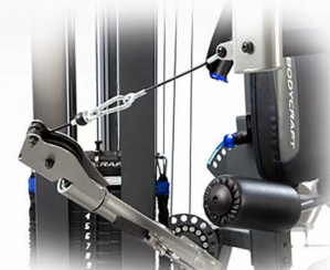
UNIQUE DOUBLE UP FEATURE INCREASES RESISTANCE FROM 1:1 TO 1:2 - UP TO 400 LBS RESISTANCE
